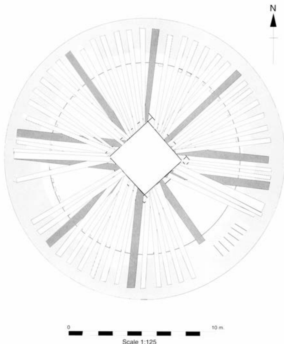
Figure 3.16: The Keep: reconstruction of cannon deck timbers
